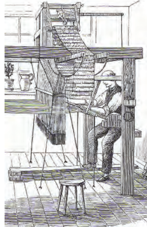
Jacquard's loom, the first use of punched cards to control machine function
