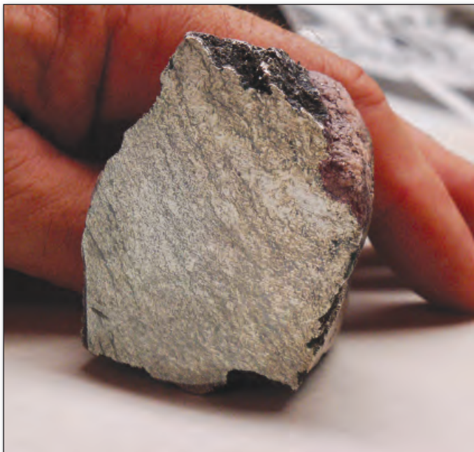
Slice of metallic silver from a Mollie Gibson Mine mass; the adherent material at upper right on the sample is pink barite, a characteristic association of Aspen ores. Aspen nuggets were believed formed by reduction of sulfide ores in underground water channels
