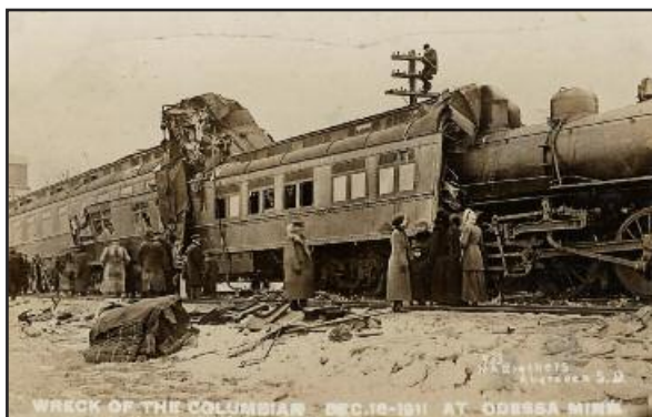
This postcard shows telescoped cars of the “Columbian”. Ten were killed and ten more seriously injured in 1911 when the second section of train No. 18, the Columbian from Seattle, ran into the first section, which had been stopped at a signal
