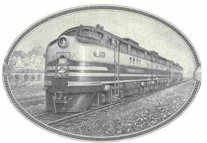
Image of locomotive 901 engraved by Security Banknote Company. Well-known from 1950s-era Western Pacific Railroad Co. stock certificates, this diesel was a Model FTA, 1350 horsepower machine built by Electro-Motive Corporation. It was put into service on Nov 29, 1941.
