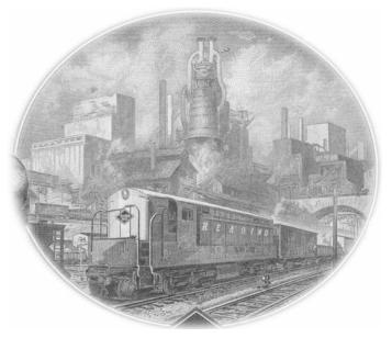
This ABNCo image appears on late-date Reading Company stock certificates. It represents an unnumbered 1400 horsepower H24-66 "Train Master" diesel built by Fairbanks-Morse sometime between 1953 and 1956. The headlight arrangement suggests the locomotive that was the subject of the engraving was probably numbered above #850. None of the existing Reading photos show this exact shape of handrail, so the artist may have modified it slightly.
