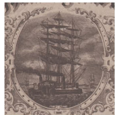
Lightering is the transfer of cargo from an ocean-going ship to a small vessel, thereby reducing its draft and permitting it enter a harbor. Here two steam-driven lighters bracket a threemasted sailing vessel.
