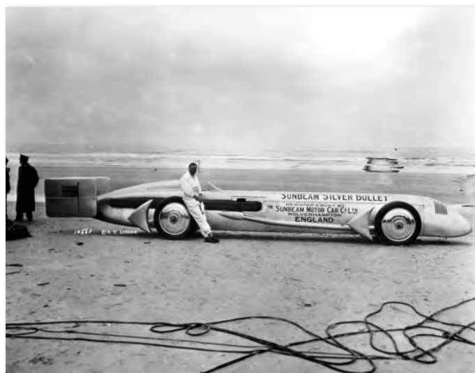
The Sunbeam Silver Bullet, built in 1929 and powered by two Sunbeam 2,000hp supercharged V12 aero engines, failed at Sunbeam's last attempt at the land speed record
