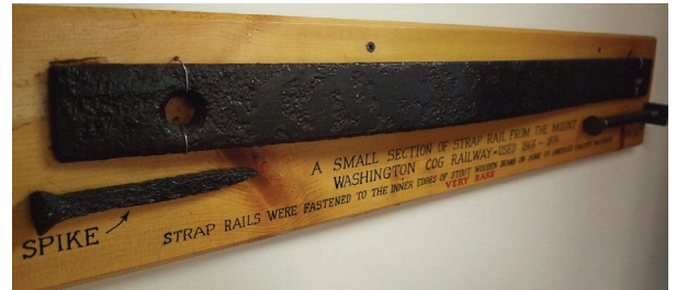
The earliest rails were simply lengths of timber. A thin iron strap was affixed to the top of the timber rail to protect it from wear, as shown in this on-line image of strapping used on the Mt. Washington Cog Railway in New Hampshire 1866 - 1868. This saved money as wood was cheaper than metal. The system had the flaw that every so often the passage of the wheels on the train would cause the strap to break away from the timber. The problem was first reported by Richard Trevithick in 1802. The use of strap rails in the United States led to passengers being threatened by "snake-heads" when the straps curled up and penetrated the carriages
